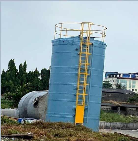
PP FRP STORAGE TANK WITH TAPER BOTTOM SLOPE- 50 KL- FOR FOSROC CHEMICAL LTD
